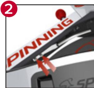
**STEP 2:** Using a wrench, carefully remove the two bolts supporting the brake pad (indicated with red arrows). Remove the old brake pad assembly.
