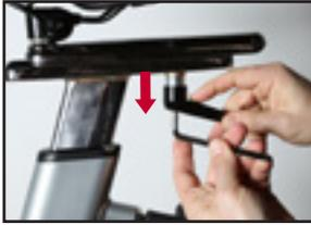
3. Position the lever straight back, then use a 6mm allen wrench to secure the bolt while pulling down on the lever (as shown left).
