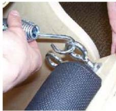
1. Each spring has one end which is a “closed loop” and one which is “open”. Attach the “closed loop” of each spring over one of the spring posts mounted on each side of the inside rear of the chair.
